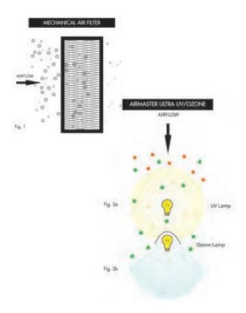
Air purifiers, on the other hand, actually sterilize or kill most contaminants. Both UV and ozone are purification methods. In the Airmaster Ultra, when air passes within the UV light zone (Fig. 2a), most airborne bacteria and molds are killed or sterilized. From there, the air passes by the ozone lamp (Fig. 2b) where odors are neutralized. The process happens continuously and silently as your heating/cooling system runs, and there are no messy filters to change.
